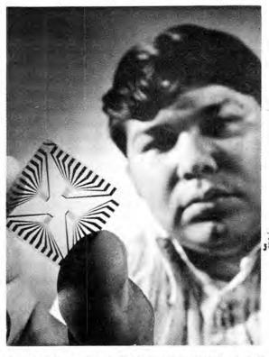
GEORGE LAGUNA (2521) displays prototype of a ceramic light gate. An array of 256 of these tiny shutters will serve as an information input device — page composer — for an optical (holographic) computer memory.
